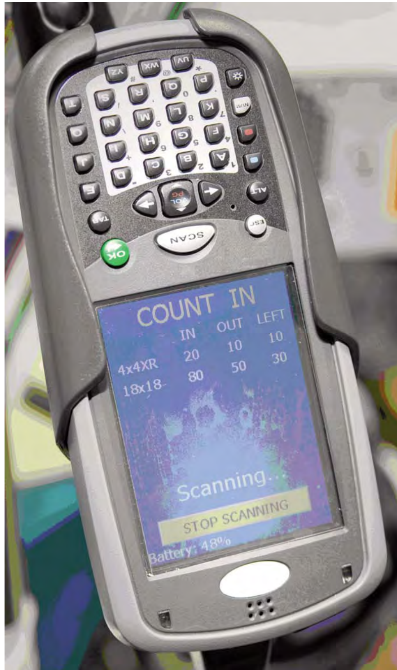
Figure 2. The data-matrix scanner shows the type of and the number of sponges still on the sterile field and the number of sponges that have been removed from the sterile field.
